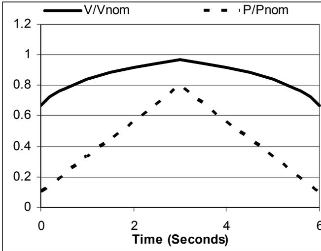
**Figure 5-2 Fast Ramp Voltage and Power Curves.** Not shown is the dwell time at the 800 W/m<sup>2</sup> condition and at the beginning and end of the ramps while the MPPT stabilizes.
