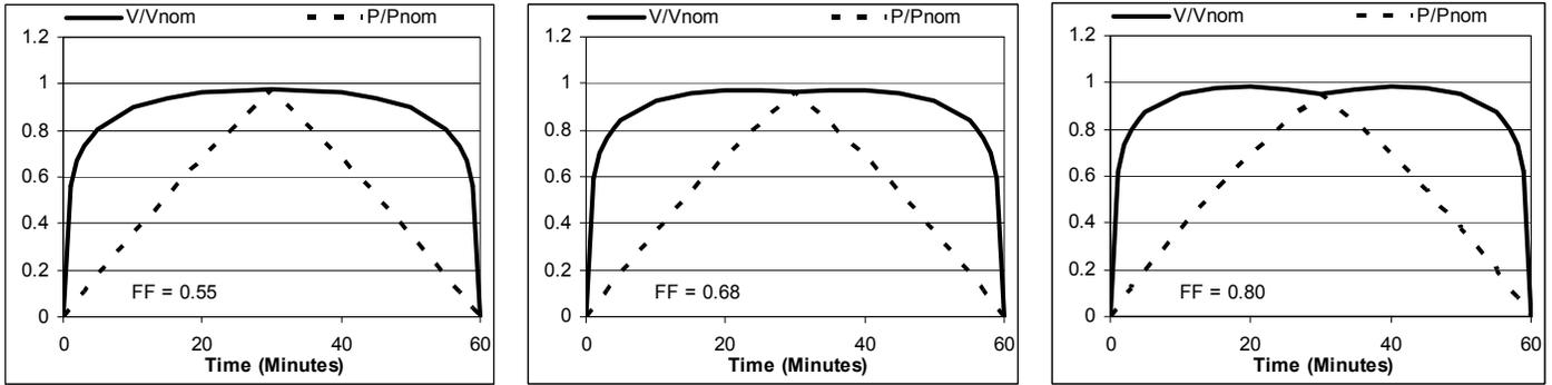
**Figure 5-1 Slow Ramp Voltage and Power Curves.**  $V_{REF}$  is the inverter nominal input voltage and  $P_{REF}$  is the inverter rated input power. The three curves represent the three PV technologies listed in Table 5-6.
